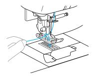
Pull out about 10-15 cm (4-5 inches) of the bobbin thread under the presser foot toward the rear of the machine.
